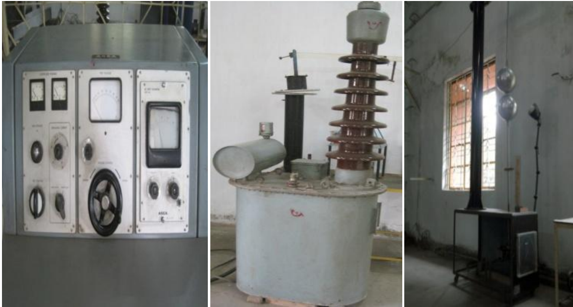
Fig: 3.1 Control Setup, Transformer, Sphere Gap
