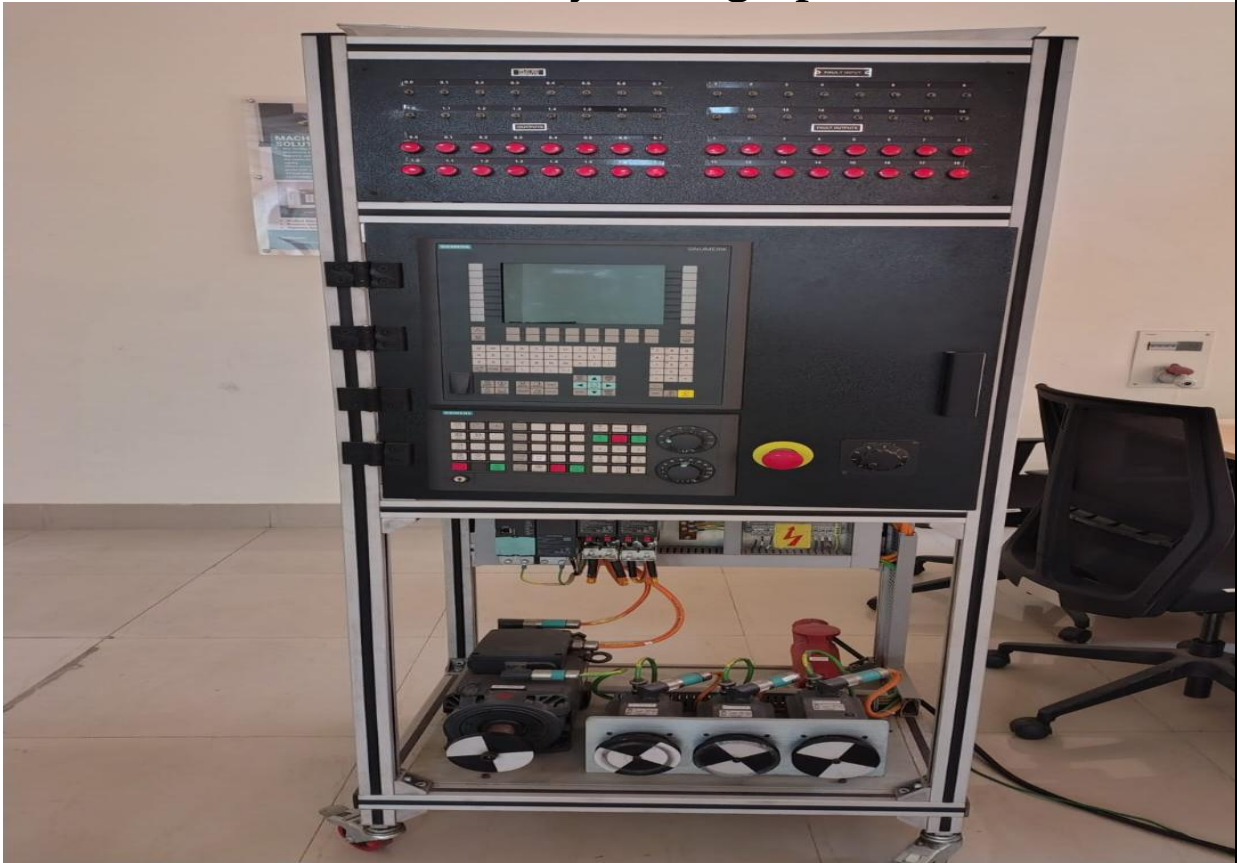
840D SL KIT with Sinutrain Software
